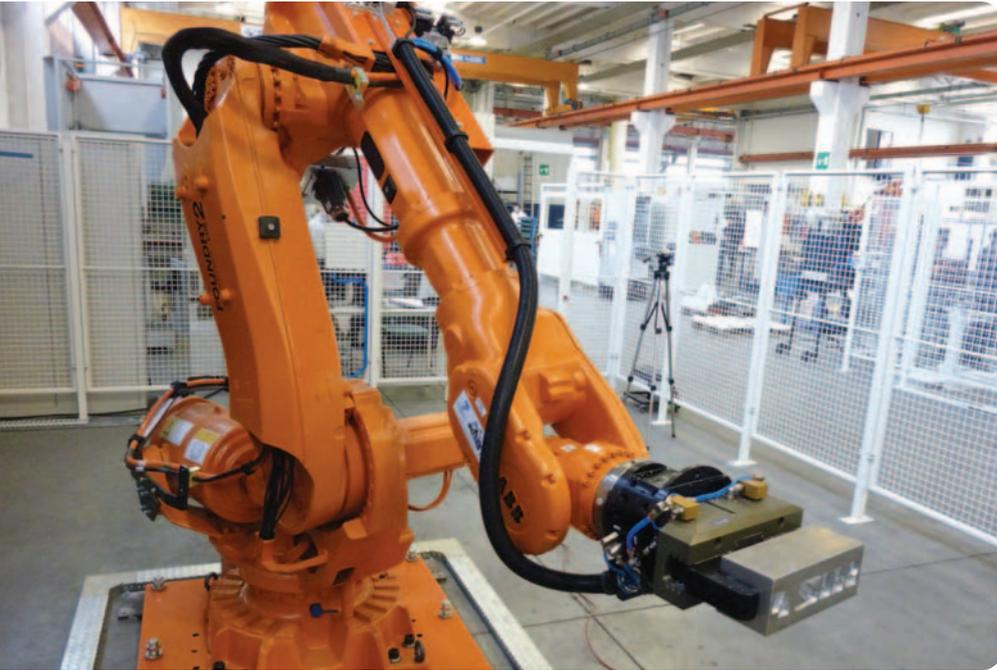
kinematic profile, the system cannot produce collision-free toolpaths, automatically avoid 'singularities' or identify reachability. Also, the redundancy of certain robot axes is not used in support of potential optimisations.
